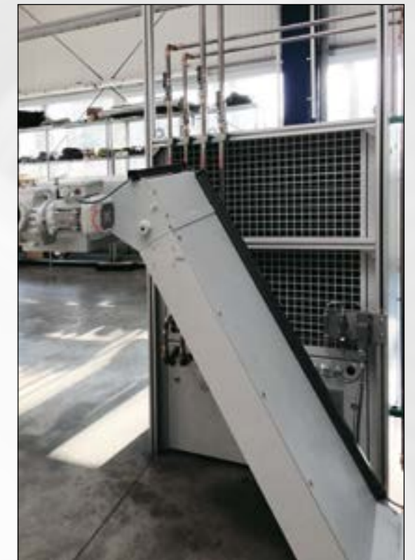
Cooling device and chip conveyor
