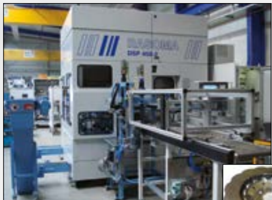
RASOMA double spindle-machining center DSP 450-2 e. g. for perforating braking discs
